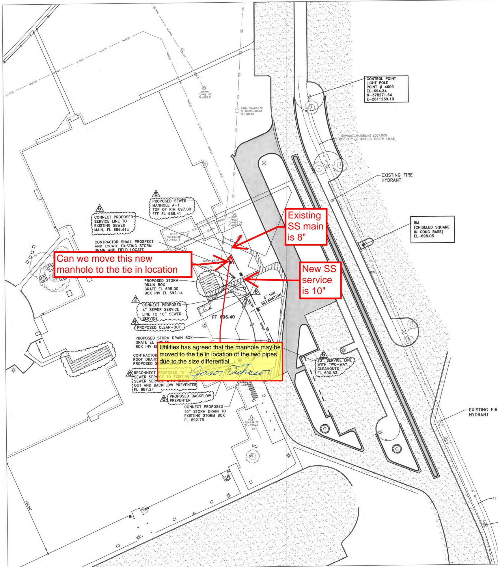
Can we move this new manhole to the tie in location
